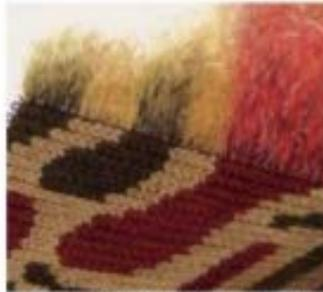
Close-up of Glenoit silver knot pile construction.
